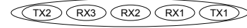
Fig. 6: In this figure, the geometrical configuration of the LORA system is shown, with two transmitting antennas and three receiving antennas. The spacing between each antenna is approximately 0.7m
