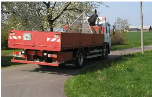
Fig. 9: The target truck with corner reflector on the roof.
