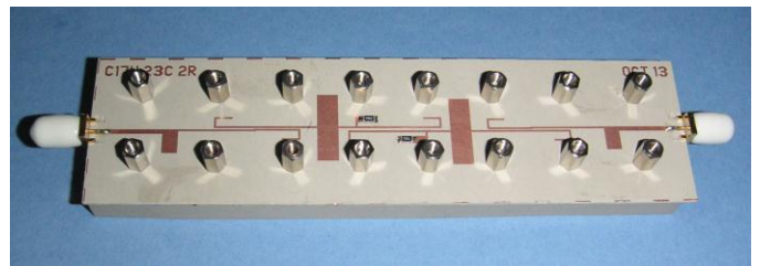
Fig. 12. The second filter, with cover removed. The 8 mm high posts are used in lieu of side walls. The first filter required neither posts nor cover. The cover is copper-clad PCB, with the same dimensions 150 mm x 40 mm as the substrate, and holes drilled to screw it to the posts.
