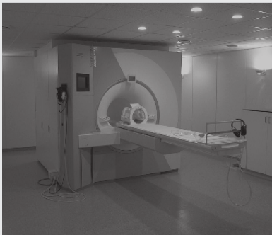
Figure 1.2 Photograph of the MRI scanner used in our experiments. The main magnetic field of this scanner is 3 Tesla.
