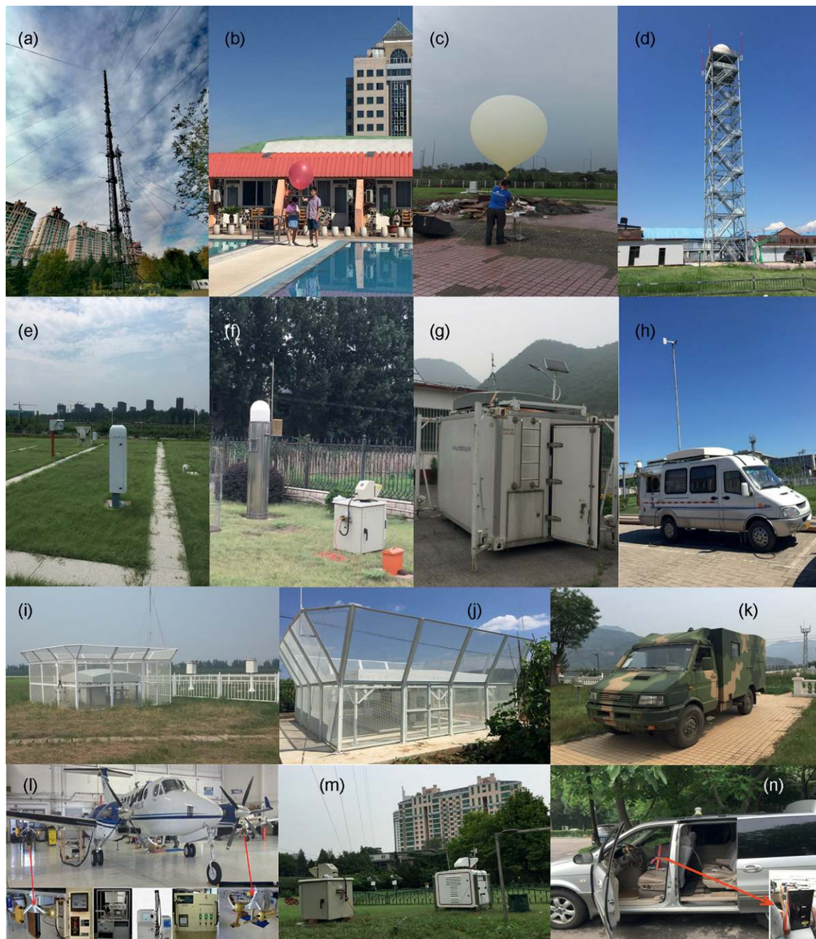
FIG. 2. Photographs of some SURF instrumentation: (a) 325-m tower at IAP, (b) small-balloon radiosonde at IUM, (c) GPS radiosonde at NAN, (d) X-band radar at SHU, (e) ceilometer at LIA, (f) mini-MPL at DAX, (g) wind profiler at SID, (h) mobile wind profiler at CHA, (i) wind profiler at SHA, (j) wind profiler at YAN, (k) wind profiler at GUC, (l) King Air airplane, (m) Doppler lidar and mini-MPL at IAP, and (n) mobile MPL (abbreviations are defined in Table ESI).
