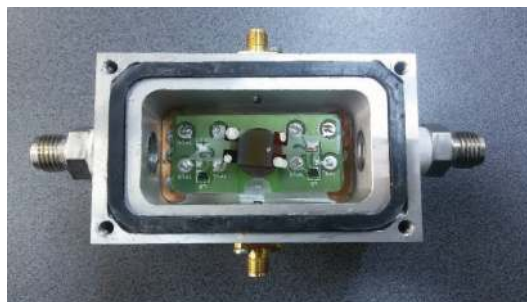
FIGURE 1: SAW S2 sensor in a test chamber.
