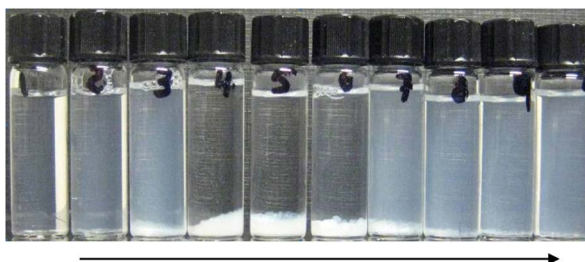
Figure 3. Typical visual effect of increasing AOT surfactant concentration on MO seeds protein solution (0.05% w/v).
