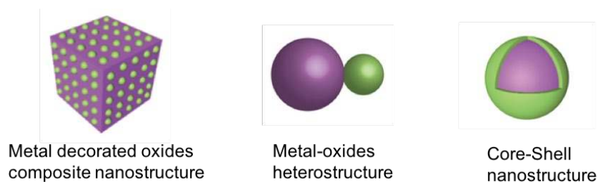
Figure 35. Schematic of metal-oxide hybrid structure with different architecture. 503 Reprinted with permission from ref 503 . Copyright 2018 Macmillan Publishers Limited.
