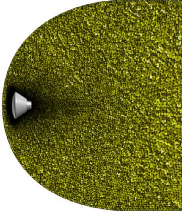
Figure 4: An example of computational grids around ESA ARD for plasma flow simulation.
