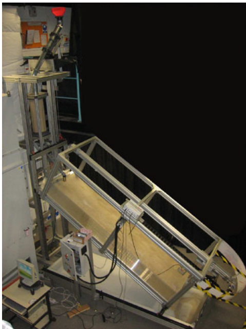
Fig. 1 Photograph shows the experimental set up. The cylindrical hopper of sand, the rough inclined plane and the instruments used to measure the flow are all supported by an aluminium framework
