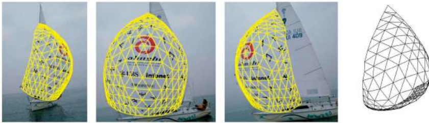
Fig. 9. Three-dimensional model of the spinnaker overlaid on the three images used to compute its reference shape and texture. In each image, we specified 10 correspondences with a CAD model of the spinnaker and used them, along with automatically detected silhouettes, to deform it. We assume that the spinnaker did not deform in these images because they were taken in quick succession by a chase boat.
