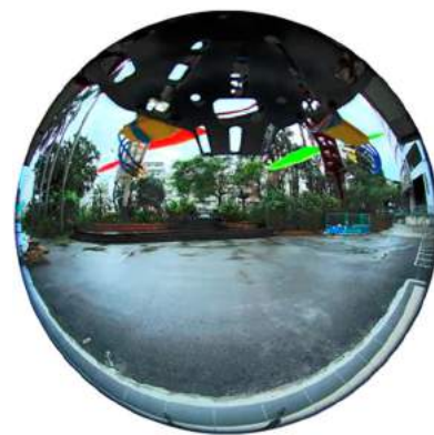
Figure 4. Unwanted obstruction caused by the body of drone in the image taken with fish-eye lens.
