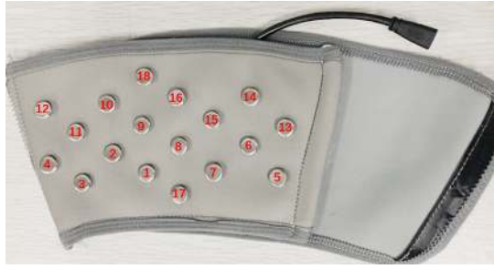
Fig. 1: The electrode cuff for sEMG signal recording. Sixteen monopolar channels record the differential voltage between electrodes 1-16 and electrode 17. Electrode 18 provides the bias voltage to eliminate DC offset.
