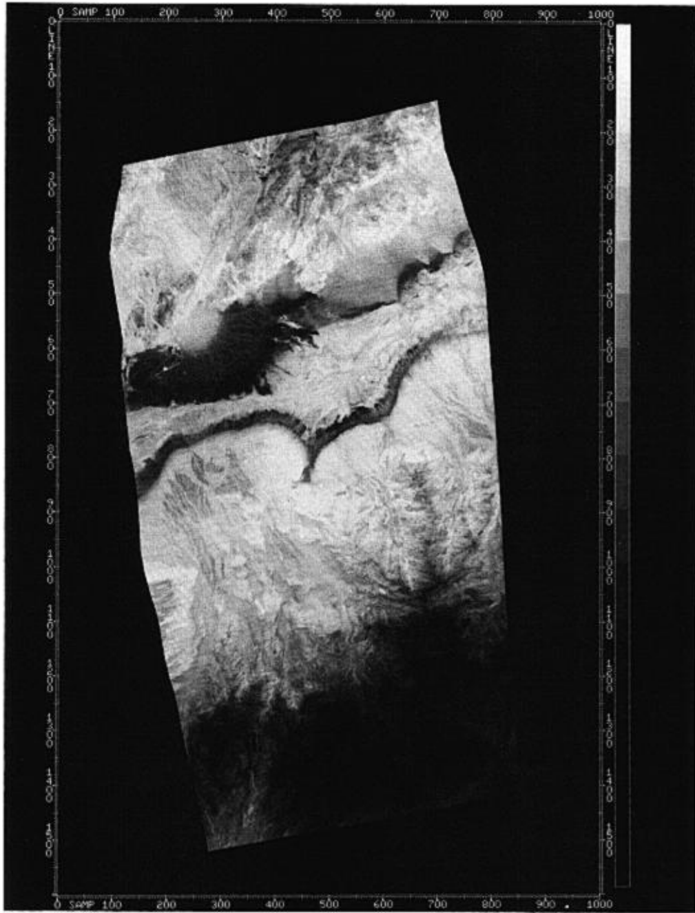
FIG. 5. Night temperature image, registered to the Landsat TM image. Bright is hot.
