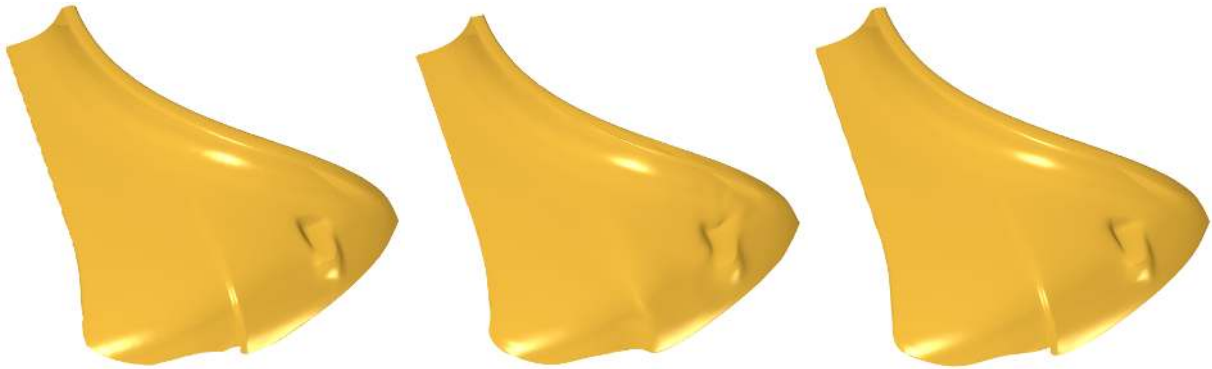
Fig. 10. Fitting a car part (left) by a cubic B-spline surface with 20 \times 30 control points and a FS parametrization (center); the result can be further improved with SDM (right).
