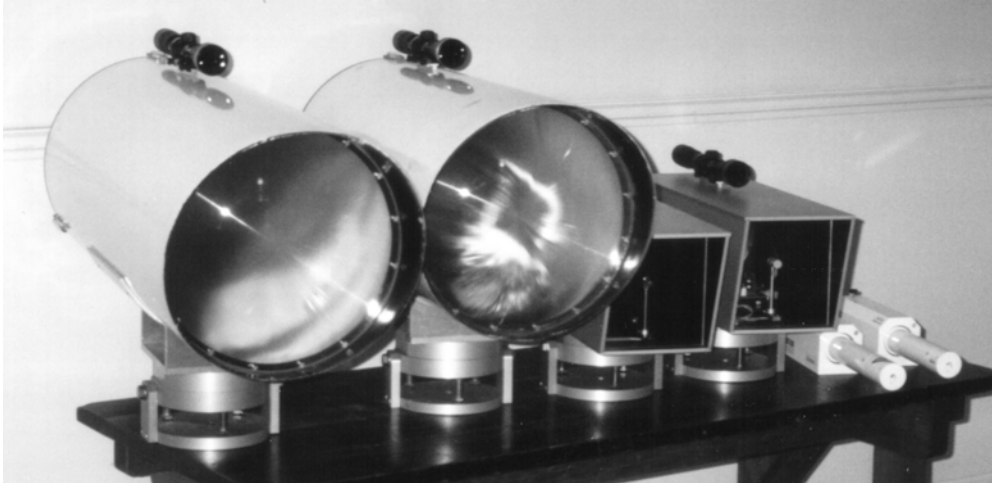
Figure 1.3: From left to right the transmitter and receiver unit of the XLAS, the LAS and the laser scintillometer from Scintec (SLS20, Scintec, Atmosphärenmesstechnik GmbH, Germany).
