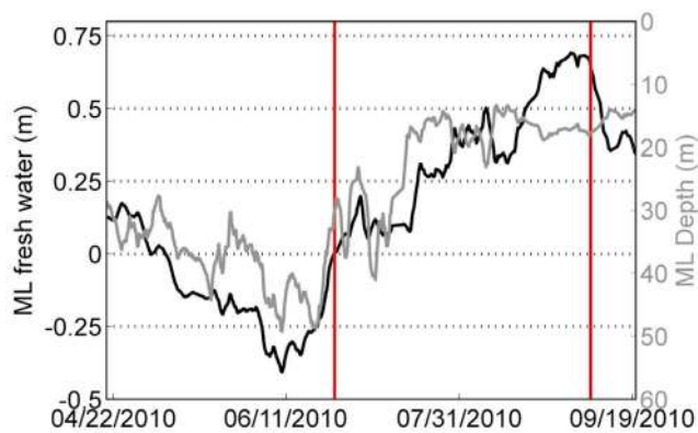
Figure 5. Change in freshwater content of the surface mixed layer over the course of the IBO drift (calculated relative to freshwater content on 25 June 2010 at the onset of the melt season) (solid curve). Mixed-layer depth defined as that point where the potential density relative to 0 dbar first exceeded the shallowest sampled density by 0.01 \text{ kg m}^{-3} (shaded curve). The mixed-layer salinity was taken as the mean over the mixed layer and was assumed to remain uniform from above the top depth (7 m) sampled by the ITP. Vertical red lines mark the start and end of the melt period.
