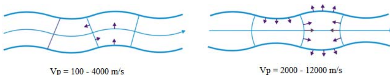
Figure 18. Pictorial representation of Lamb wave modes: (left) antisymmetric mode and (right) symmetric mode. Typical wave speeds, V_p , are shown below each sketch.
