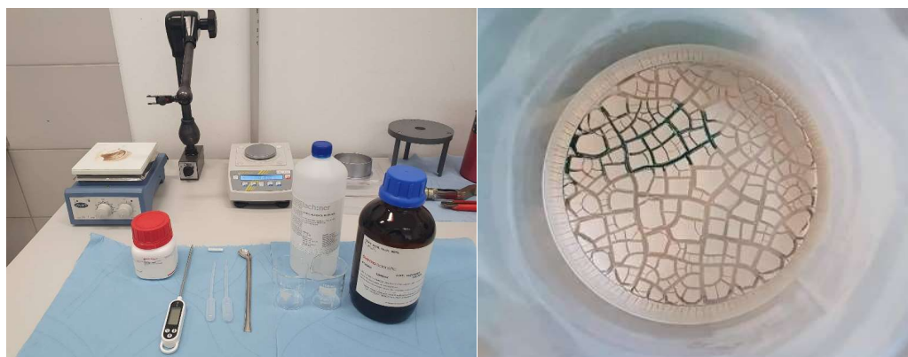
Figure 2. Tools and materials used for surface modification are on the (left). On the (right), the nanopowder was obtained at the end of the surface modification.
