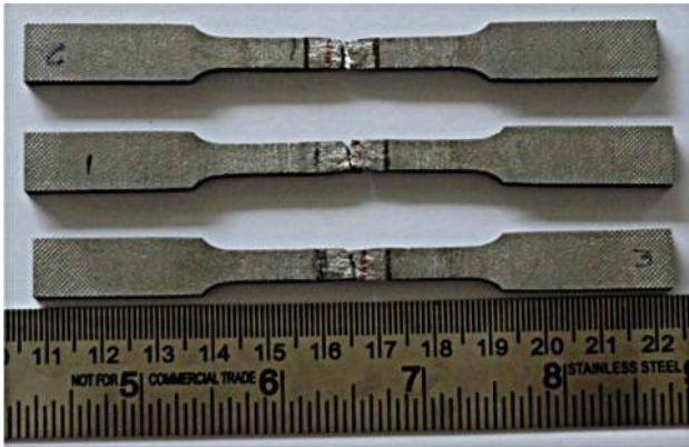
Figure 5. Tensile fractured laser shock peened specimen.
