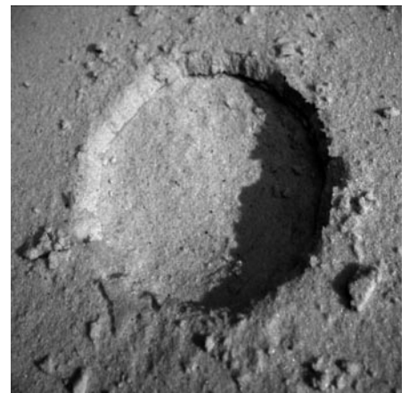
Fig. 5. A 10-cm-sized laboratory hypervelocity impact crater made as an analog of Wild 2's flat-floor craters. The crater was made with a 3.2-mm ceramic projectile impacting a porous target at 2 \text{ km s}^{-1} .
