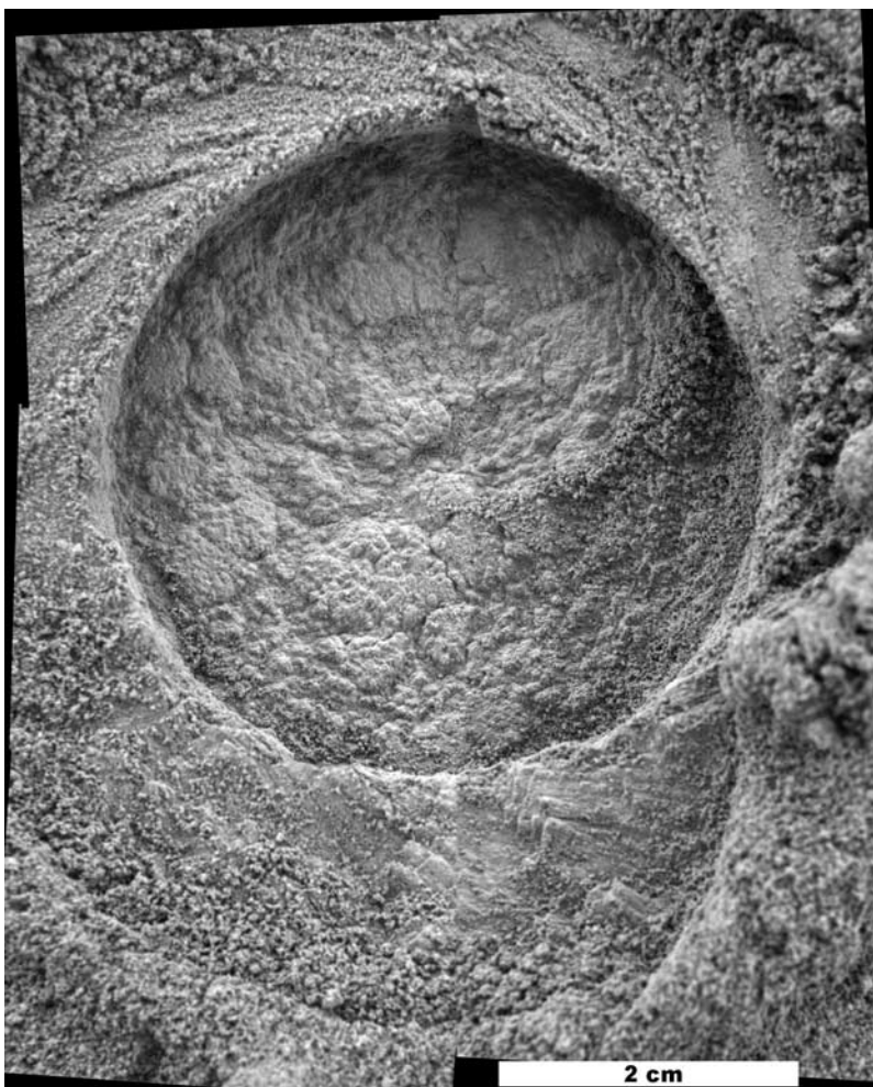
Figure 17. MI mosaic of target Holman_3, taken after RAT grinding on sol 178 when target was fully shadowed. Note unusual cauliflower-like texture within RAT hole.
