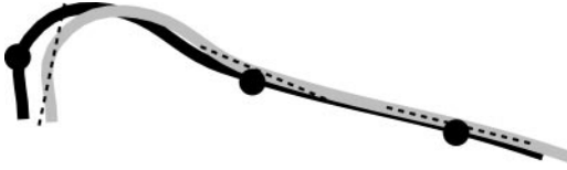
FIG. 6. Minimizing the distance from a point to a plane allows the left pair to pull the surfaces into alignment without the other pairs resisting tangential sliding.
