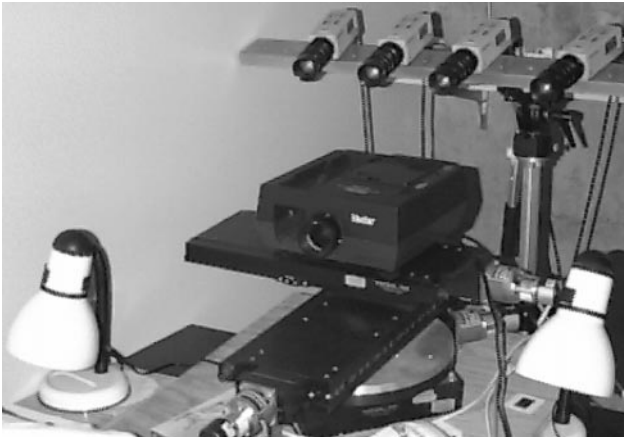
FIG. 1. The scanner hardware: four video cameras, a slide projector on a turntable, and table lamps.
