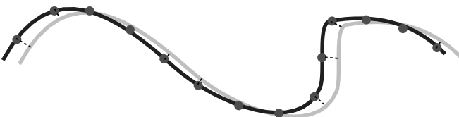
FIG. 5. If many of the paired points do not correspond to the same surface points, many seemingly good pairs (short distances) resist motion in all directions.
