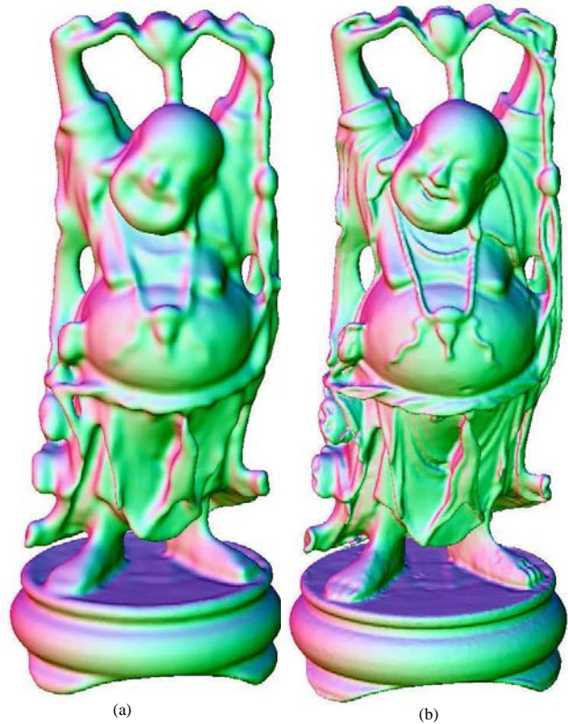
Figure 20: Surface reconstruction at varying levels of detail. (a) Octree level 6. (b) Octree level 8.
