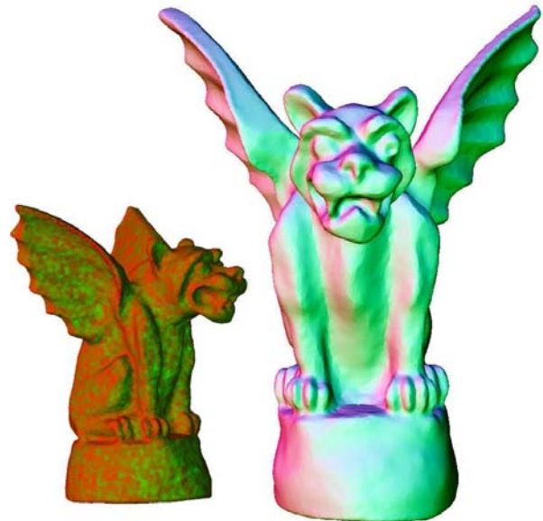
Figure 1: Our noise-tolerant surface reconstruction system. The noise rate is 0.7% of the object size. The side view of the gargoyle shows the fitting error map. Red color indicates larger fitting error.
