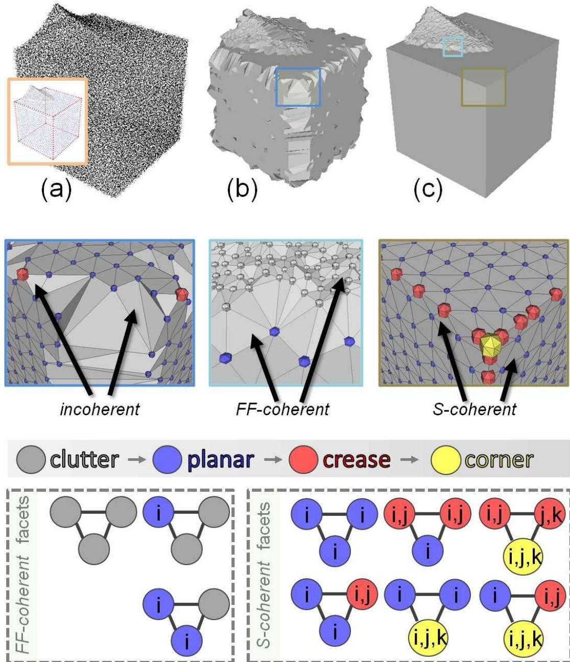
Figure 9: Facet coherence. Starting from a noisy input point set (a, depicted with its structured point set in the closeup), we reconstruct two models: one with many *incoherent* facets (b), and one with all facets either *FF-coherent* or *S-coherent* (c).  $i$ ,  $j$  and  $k$  each corresponds to a primitive index in the *FF-coherent* and *S-coherent* facet description (bottom).
