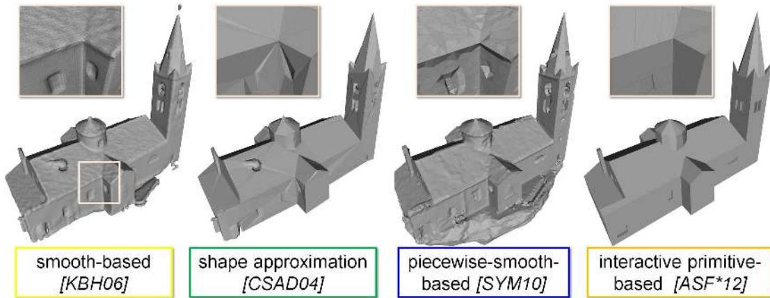
Figure 2: *Church* model reconstructed by different families of methods. Note that the shape approximation has been realized from the smooth model (left). The primitive-based model (right) has recovered the building structure, but by requiring 15 minutes of snapping-based user interaction.
