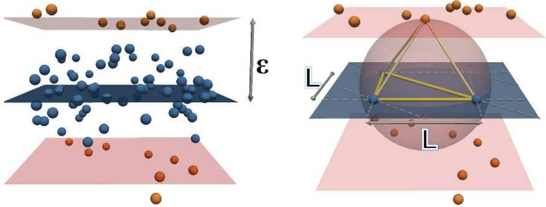
Figure 4: Plane anchor sampling. Inliers to the planar primitive (blue dots) are removed from the point set and new points are created on the plane according to a 2D-grid of width  $L_p$  so that the induced facets exist in the Delaunay triangulation.  $L_p$  is determined in function of the fitting tolerance  $\epsilon$  so that circumspheres of the induced facets stay inside the  $\epsilon$ -domain of the primitive.
