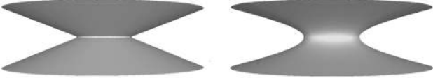
Figure 5: Reconstruction with linear interpolation (left) and a natural cubic spline (right) for the corresponding speed functions. The inputs are three circular contours, two large ones at the top and bottom and a smaller one at the center.
