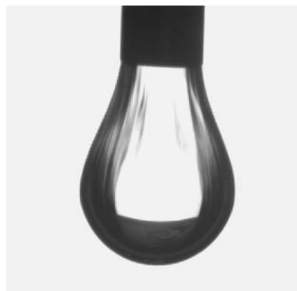
Figure 9. Image of a pendant drop from a 0.1 wt % saponin solution after fast surface compression with \alpha = 12\% . The wrinkles in the region of the elongated drop neck indicate the compressed nonhomogeneous adsorption layer.
