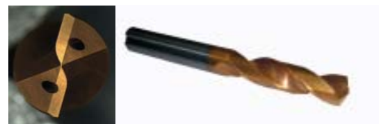
Figure 3. Photograph of Twist drill (make Sandvik) used in the tests
