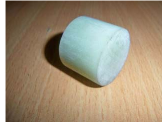
Figure 1. Photograph of the GFRP rod manufactured by pultrusion process
