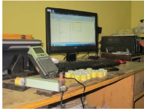
Figure 7. Photograph of surface roughness tester used for measuring R a values
