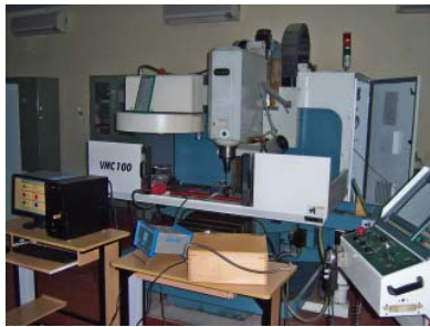
Figure 4. Photograph of the experimental setup used for drilling GFRP composite rods
