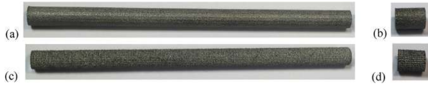
Fig. 1. Full size views and cut parts of Ti_S (a,b) and Ti_R (c,d) fibers.
