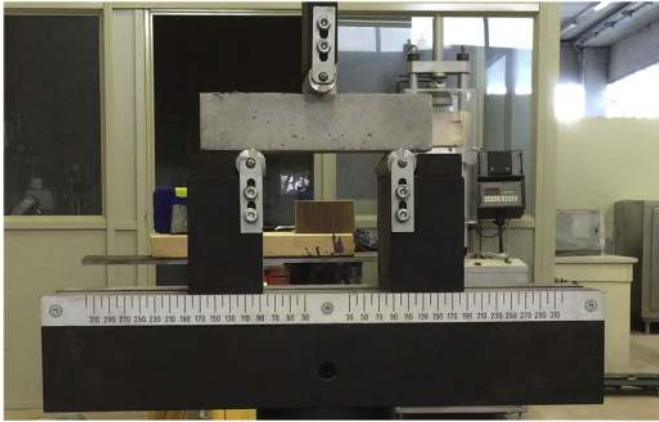
Fig. 2. Setup of short-beam shear tests.
