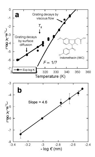
FIG 2. (a) Decay constants K of 1000 nm gratings of IMC liquids and glasses. (b) K vs. grating wavelength at 295 K.
