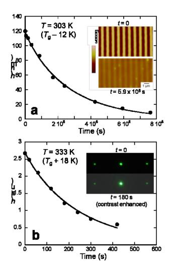
FIG 1. Decay kinetics of 1000 nm IMC gratings. (a) Grating amplitude h vs. time at 303 K measured with AFM. Inset: AFM images at 0 and 5.9 x 10<sup>5</sup> s. (b) h vs. time at 333 K measured with diffraction. Inset: Diffraction patterns at 0 and 180 s. The side spots are from first-order diffraction. Contrast is enhanced in the 180 s pattern to make the diffraction spots more visible.
