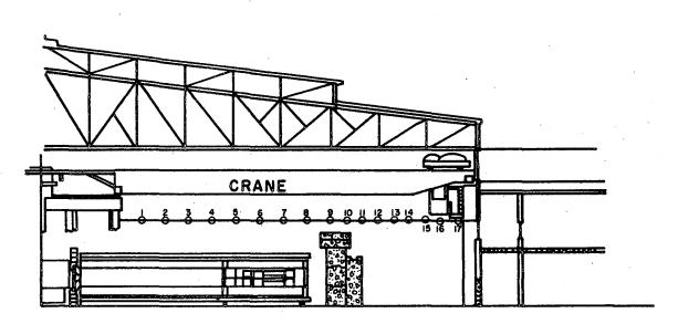
Fig. 6. Section view of Bevatron and building through Bay 20 showing radial positions of indium foils.
