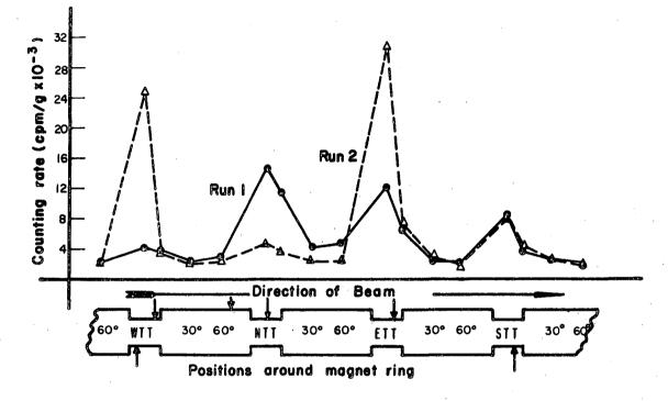
Fig. 5. Counting rates at various positions around Bevatron magnet ring. (Actual activity of moniter foils, Run 1-1850 cpm/g; Run 2 - 4480 cpm/g.)
