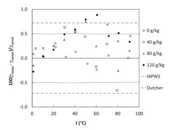
FIG. 1. Percent deviation of surface tension measurements of ACS water and aqueous sodium chloride from the IAPWS correlation<sup>15</sup> and Dutcher's correlation<sup>31</sup>, respectively, along with the uncertainty in the IAPWS correlation and average absolute percentage deviation in Dutcher's correlation.
