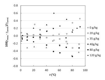
FIG. 3. Deviation of surface tension measurements for ASTM seawater from surface tension calculated by Eq. 2.
