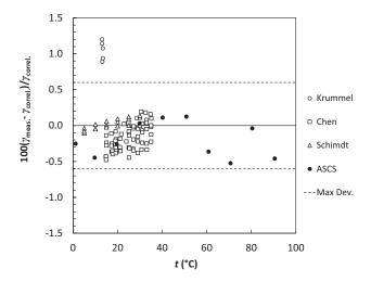
FIG. 5. Deviation of seawater surface tension data of Krummel<sup>5</sup>, Chen et al.<sup>6</sup>, Schmidt et al.<sup>7</sup> and 35 g/kg ASCS seawater measurements presented in this work from surface tension calculated using Eq. 2 along with the 0.6% maximum percentage deviation of ASTM seawater measurements from Eq. 2.
