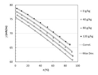
FIG. 4. Select surface tension measurements compared to the correlation given in Eq. 2 along with the maximum deviation of the correlation.
