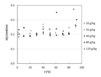
FIG. 2. Expanded uncertainty in surface tension measurements for ASTM seawater
