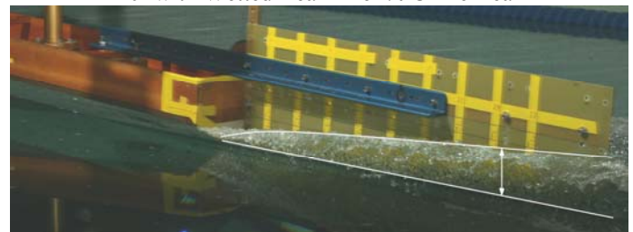
30° with Wetted Beam = 58% Chine Beam
