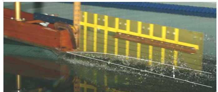
20° with Wetted Beam = 61% Chine Beam
