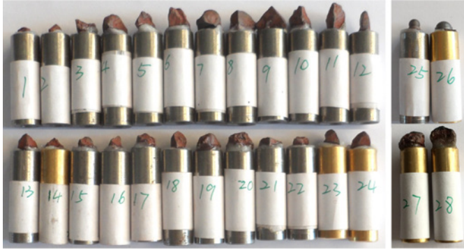
Figure 4.9: Experimental pins with SiShen particles
