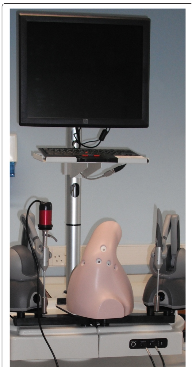
Figure 4 Virtual Reality arthroscopic simulator with haptic feedback. (Insight Arthro VR, Simbionics USA).
