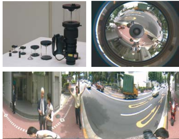
Fig. 1. Top: A hyperbolic mirror (courtesy of Accowle Corporation) mounted on top of a high-definition camera. Bottom: (Cropped) equirectangular map
