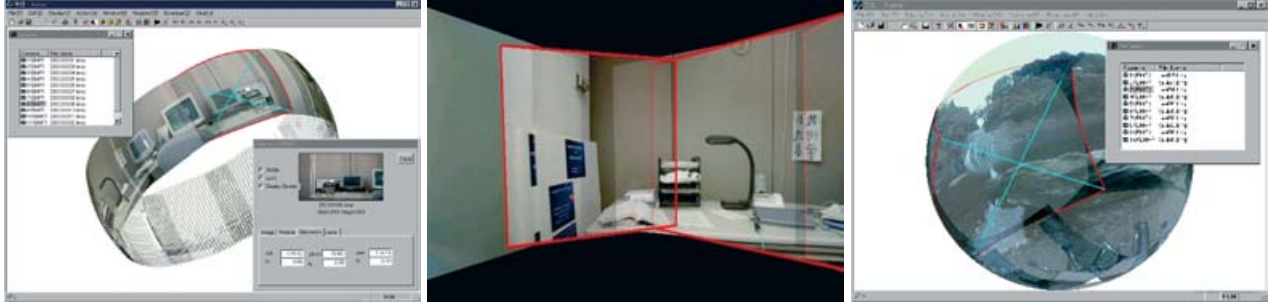
Fig. 4. Screen capture of the authoring and editing software. Left, right: project images displayed on the unit sphere. Middle: images displayed from the nodal viewpoint. Radiometric corrections are not displayed
