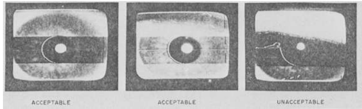
Figure 30. Operator indicators superimposed on TV image of eye as a function of threshold setting showing status of measurement. Measurement is good when pupil is properly delimited (Courtesy Whittaker Corporation).
