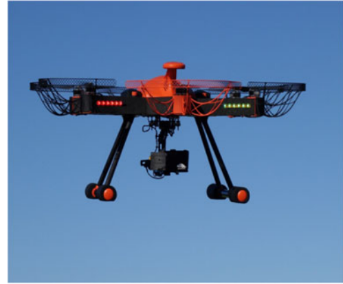
Fig. 1. PPL612-PV UAV model designed ad hoc for the extensive PV plant flight campaign.
