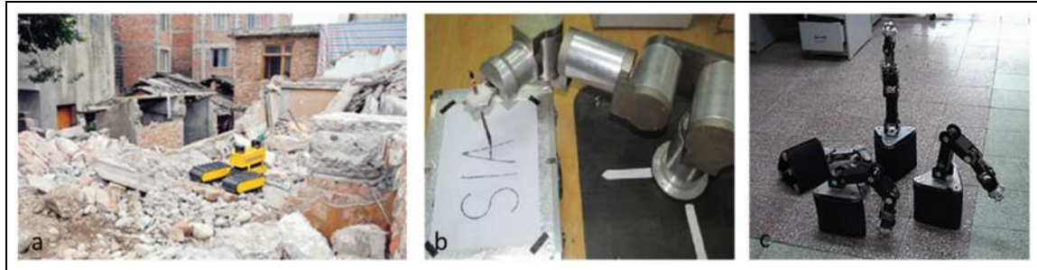
Figure 5. (a) AMOEBA-I in Ya'an earthquake, (b) SIA 6-DOF RMR, and (c) SIA wheel-manipulator robots (courtesy of State Key Laboratory of Robotics, Shenyang Institute of Automation, Chinese Academy of Sciences, China).
