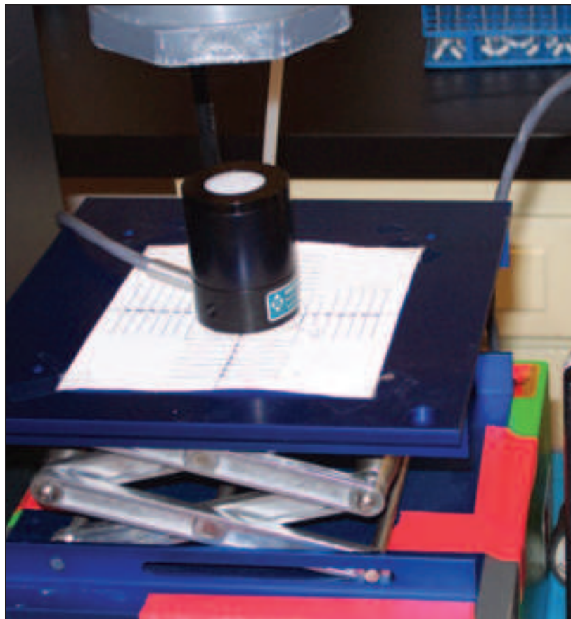
In each trial, the UV irradiance measurements obtained by radiometry were verified by examining the response of organisms of known UV response with the test apparatus and methods and comparing the inactivation achieved against reference data.
