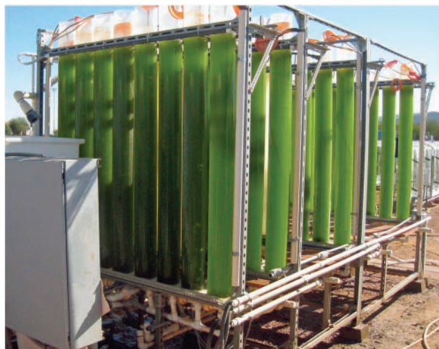
Figure 4. Portable algal nutrient recovery system cleans farm wastewater while recovering and recycling phosphorus and other nutrients. Photograph: Mark Edwards, Laboratory for Algal Research and Biotechnology, Arizona State University.
