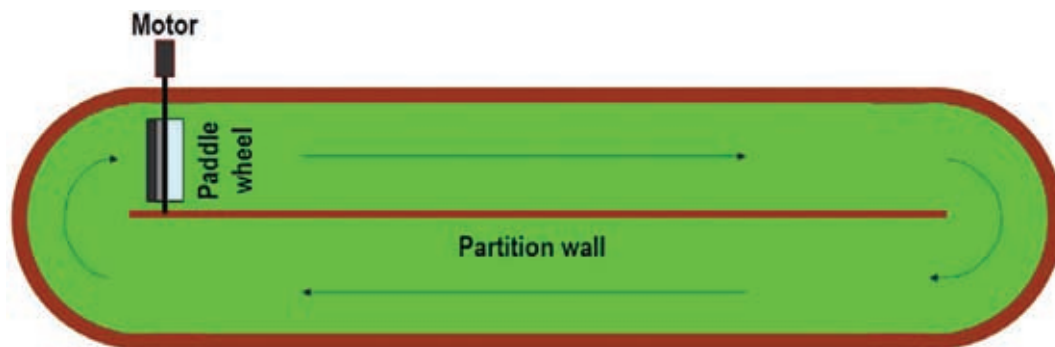
Figure 6: Schematic layout of a typical raceway pond. The salient features are i. depth 30 cm; operating depth 15 cm; Number of paddle units 1 or 2; rpm of paddles 23–36; Flow rate 50 cm/sec.
