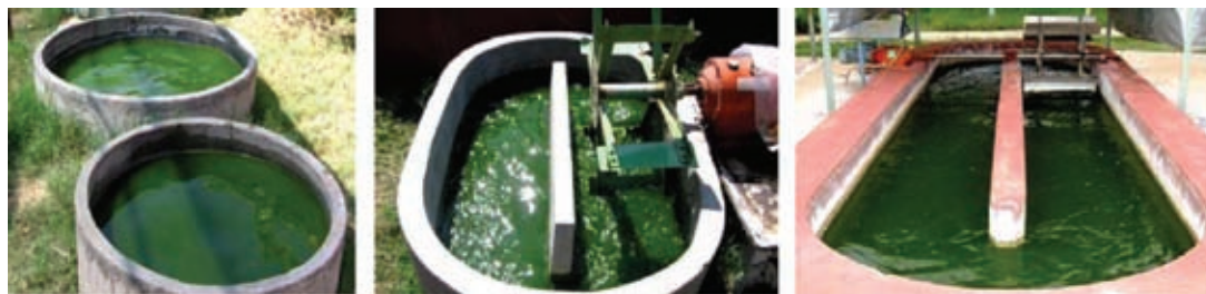
Figure 5: Outdoor open pond systems for microalgal cultivation (a) Circular Pond (b) Raceway Pond (c) Scale up raceway pond. Open outdoor raceway ponds have been used in many commercial production facilities in India. 70
