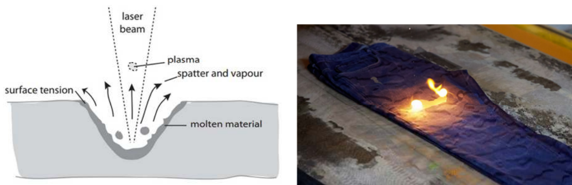
Figure 1. Laser Fading Mechanism on Denim Jeans [17, 22].
