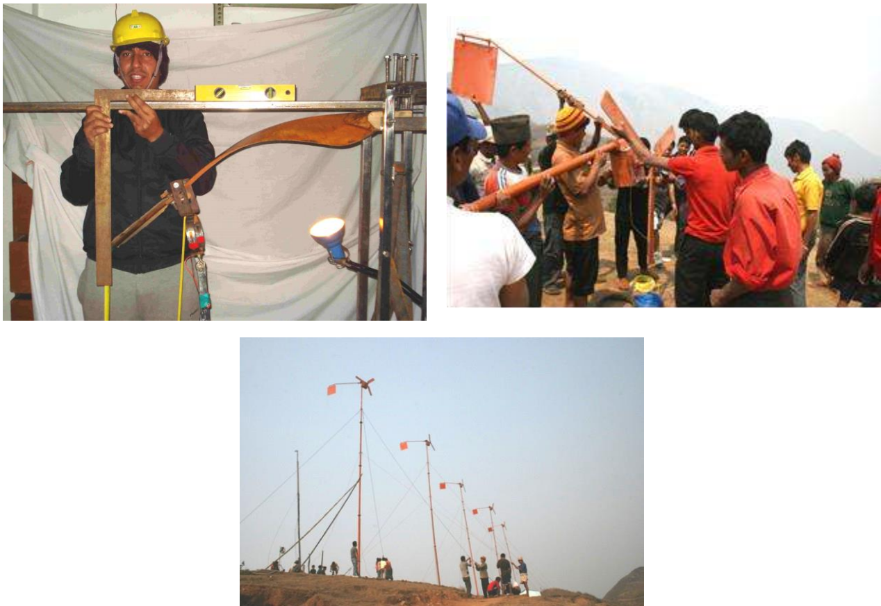
Figure 10. Locally produced wooden wind turbine in Nepal: testing and installation in Dhulikhel region. The figures are reprinted from [147] with kind permission of Elsevier.
