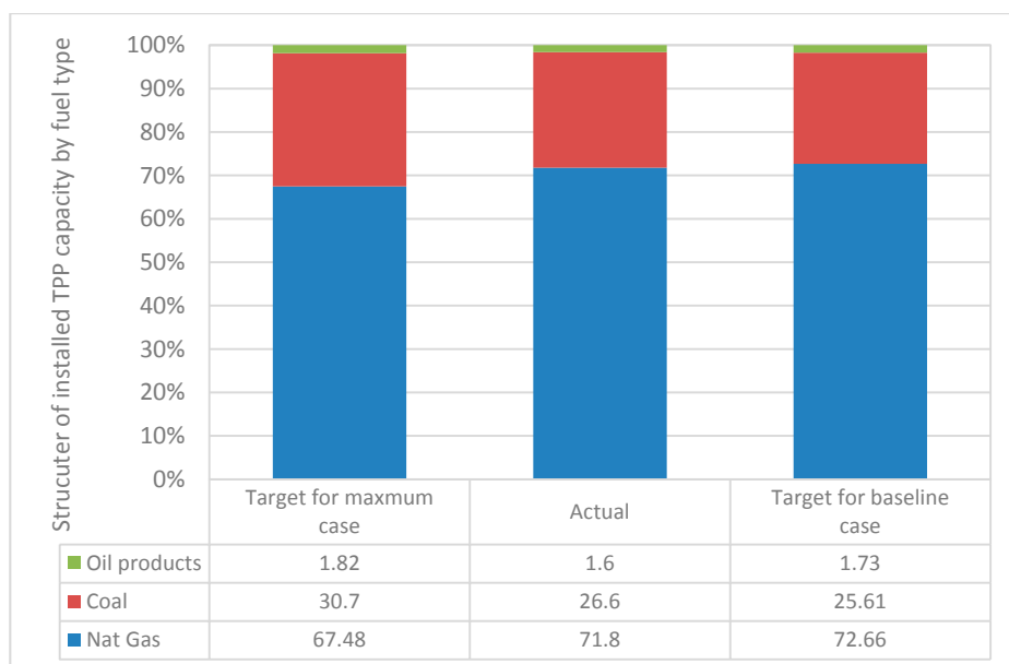
Figure 7. Actual structure of installed TPP capacity compared to projected structure for baseline and maximum cases. Source: Ministry of Energy of Russia [7], own development.
