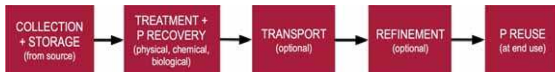
Figure 4-4. Key stages in a phosphorus recovery and reuse system: from source collection through to final reuse.
