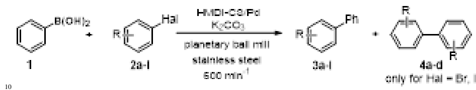
Scheme 1. Suzuki cross-coupling reaction of aryl halides in a planetary ball mill (cf. Tab. 1).
