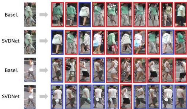
Figure 3: Sample retrieval results on Market-1501. In each row, images are arranged in descending order according to their similarities with the query on the left. The true and false matches are in the blue and red boxes, respectively.
