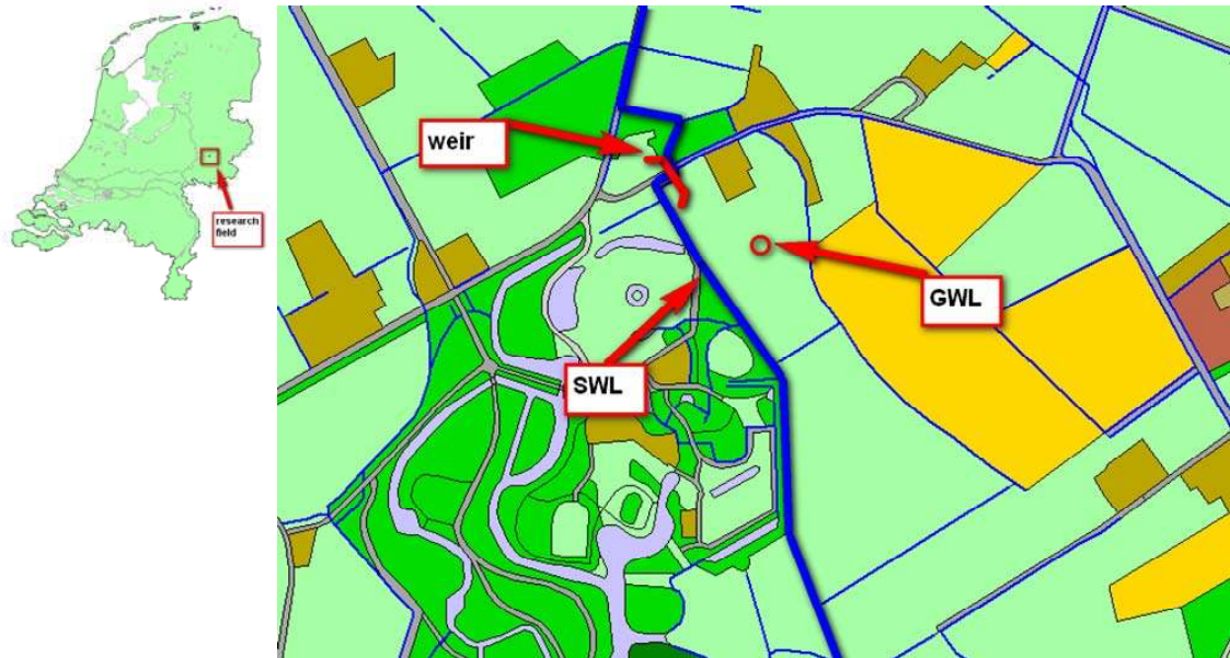
Figure 5.1 Location of monitoring site at the Wildenborch estate where groundwater levels (GWL) and surface water levels (SWL) were measured and controlled by a weir.
