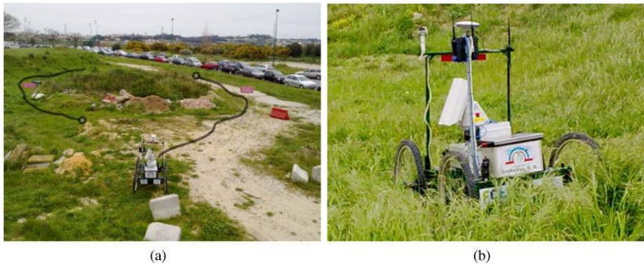
Fig. 9 Experimental site. (a) The test site overlaid with approximate paths executed by the robot in two runs. In each run, the robot started from a different position and moved autonomously to reach the specified final position, represented by a circle. (b) Situation where the difficult conditions faced by the robot are evidenced: dense and tall vegetation, which often promotes the occurrence of false positives
