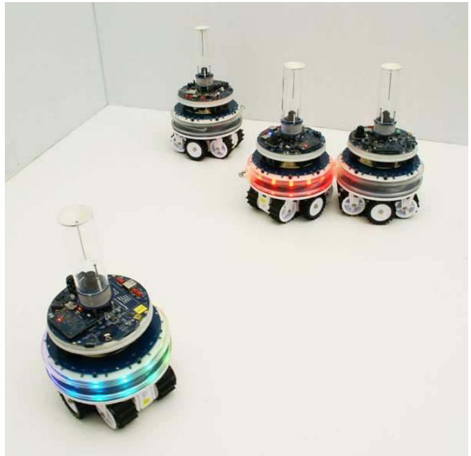
Fig. 3. The foot-bot robotic platform. The foot-bot has a differential drive system that uses a combination of tracks and wheels to provide mobility on rough terrain. Two of the foot-bots in this figure have illuminated their LED communication ring. These RGB coloured signals are detectable by the onboard cameras of other foot-bots.
