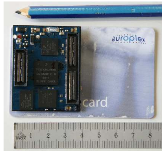
Fig. 2. The half credit card size i.MX31 main processor board.
