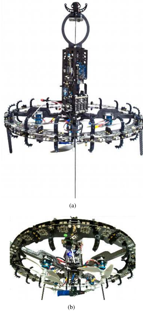
Fig. 5. The eye-bot platform. (a) The ceiling attachment system and the 24 \times 6.5 \times 6.5 cm rectangular structure housing the batteries and main PCBs. (b) The four contra-rotating coaxial rotors, the circular 3D range and bearing communication system, and the pan-tilt camera with the laser pointer.
